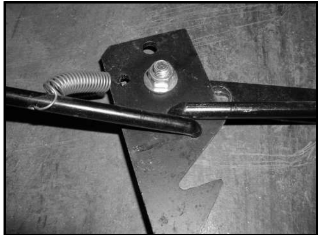
Figure 4-7 Passenger Side Catch Rods and Catch Plate
