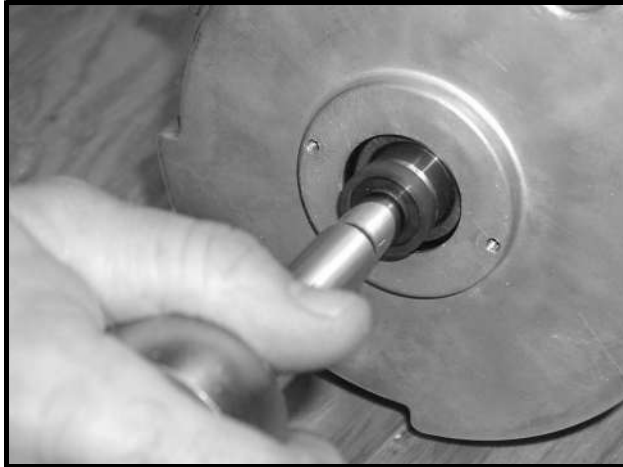
Figure 27-4 Speed Sensor Magnet
