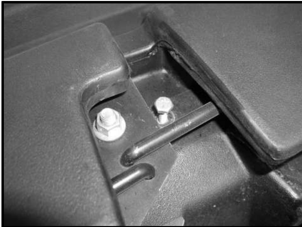
Figure 4-6 Bed Latch Link Bolt
