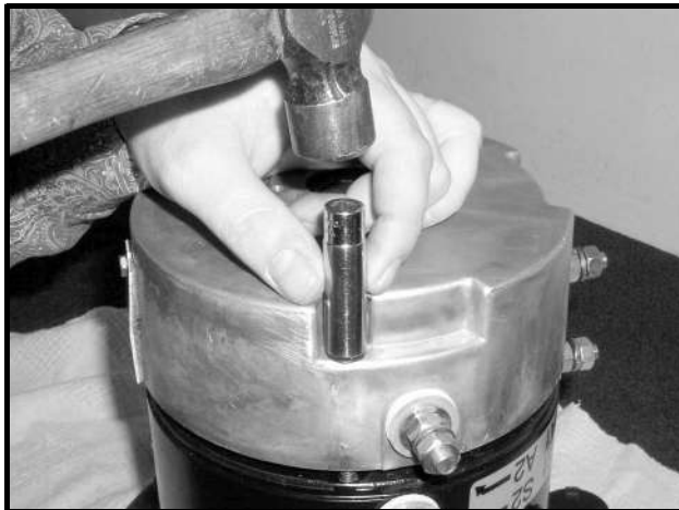
Figure 27-6 End Cap Disengagement
