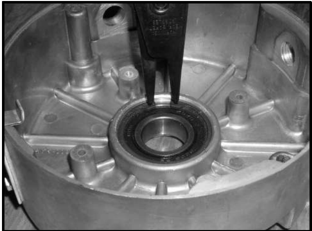
Figure 27-11 Bearing Retaining Ring
