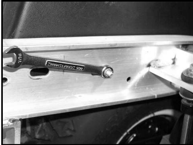
Figure 4-17 Rear Fender Frame Bolts
