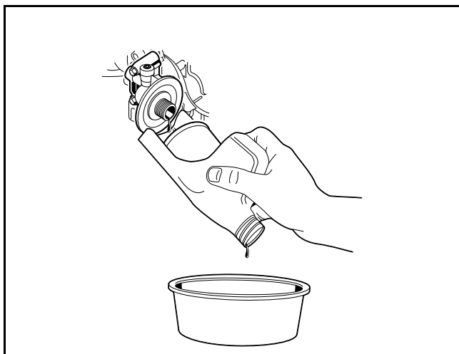
Figure 41 Remove Engine Oil Filter
