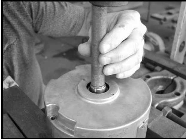
Figure 16b-8 Armature Removal
