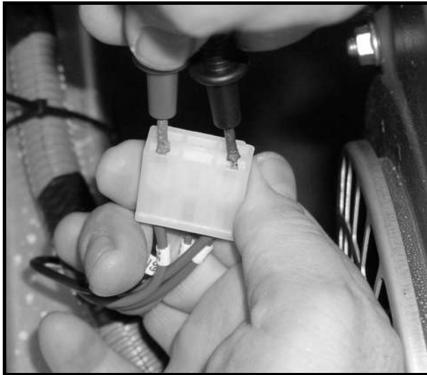
Figure 11a-21 Charge Coil Test (At Voltage Regulator Multi-Pin Connector)
