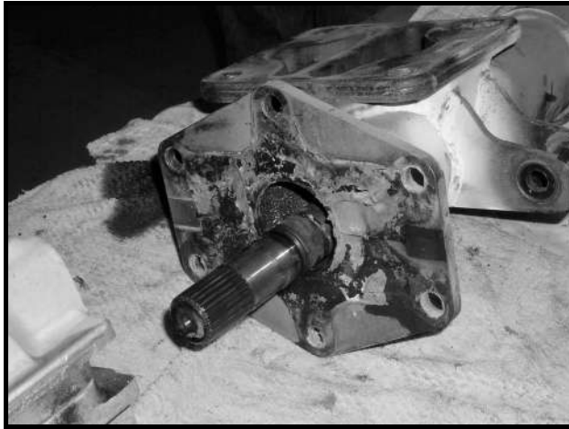
Figure 14-25 Separate Axle Tube from Differential
