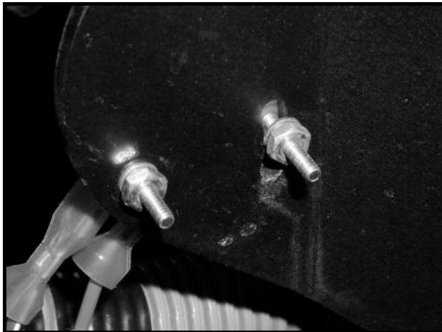
Figure 12b-8 Reverse Warning Buzzer Limit Switch Adjustment Slot
