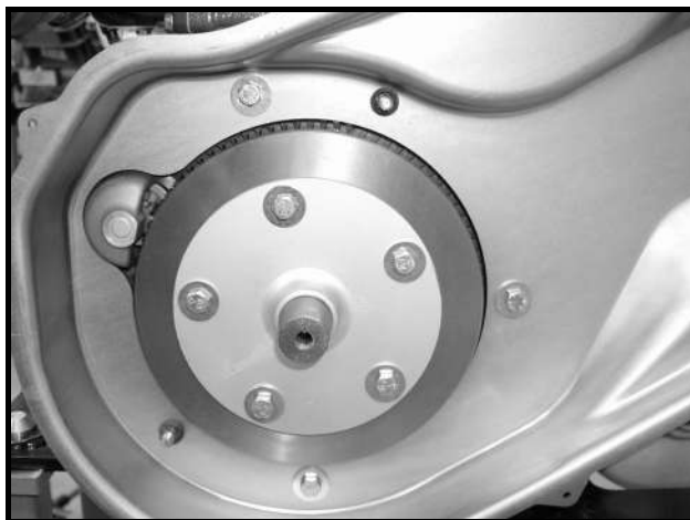
Figure 13b-40 Inner Cover Hardware on Diesel Engine
