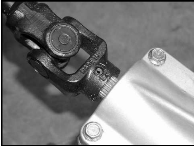
Figure 14-8 Roll Pin in Front Drive Shaft
