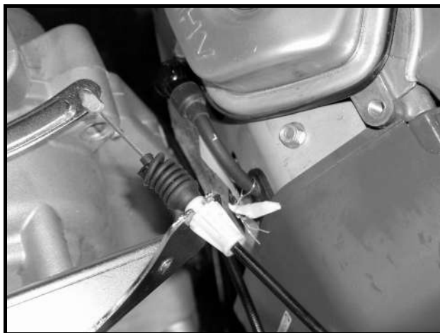
Figure 13a-20 Governor Cable on Transmission
