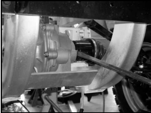
Figure 14-5 Separate Half Shaft from Differential
