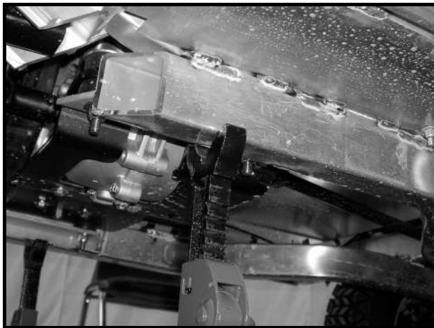
Figure 14-12 Jack Stands Under Rear of Frame
