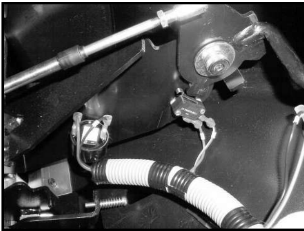
Figure 12a-6 Reverse Warning Buzzer and Limit Switch
