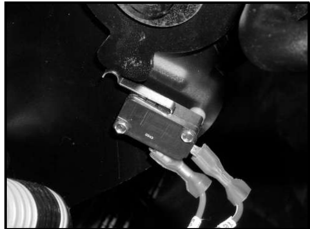
Figure 12b-9 Reverse Warning Buzzer Limit Switch (Properly Adjusted)
