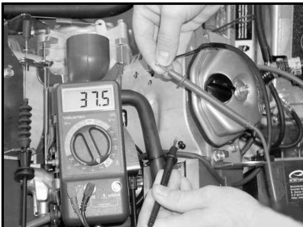
Figure 11a-26 Carburetor Solenoid Coil Resistance
