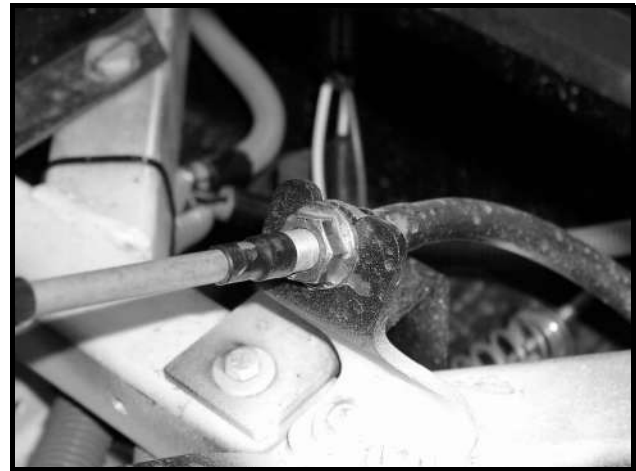
Figure 14-23 Forward/Reverse Shifter Cable Retaining Nuts At Shift Lever
