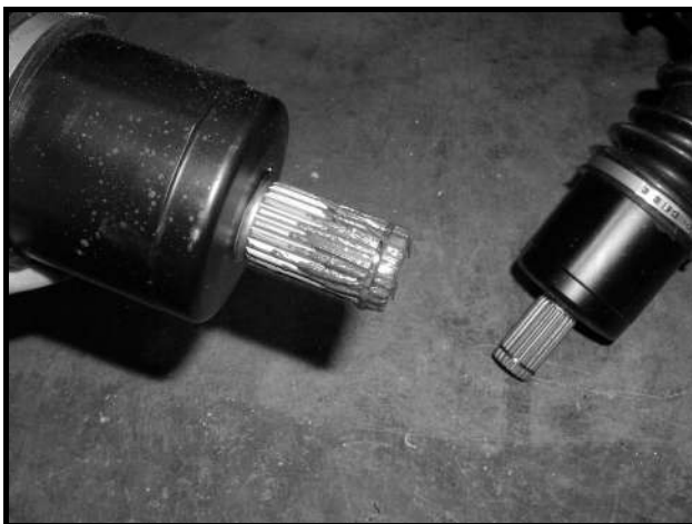
Figure 14-7 Apply Anti-Seize to Splined Ends
