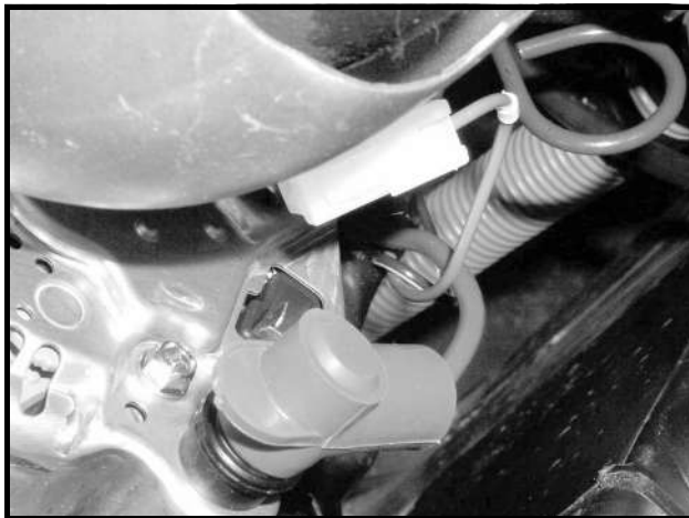
Figure 12b-11 18-Gauge Purple Wire at Alternator
