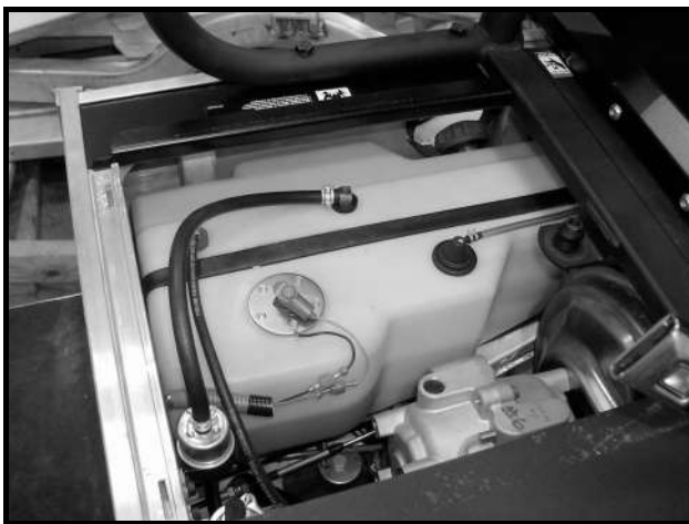
Figure 13b-18 Diesel Fuel Tank
