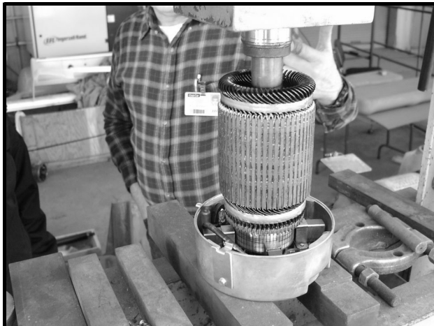
Figure 22b-18 Armature Installation
