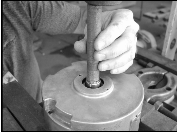
Figure 22b-8 Armature Removal
