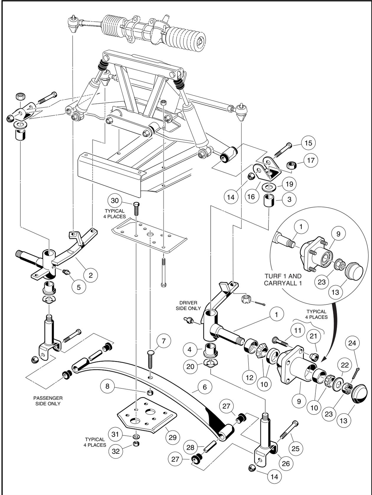
Figure 7-22 Two-Wheel Brake Vehicle – Lower Portion
