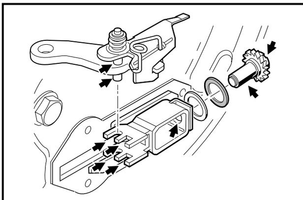
**Figure 6-10 Lubricate Adjuster**
