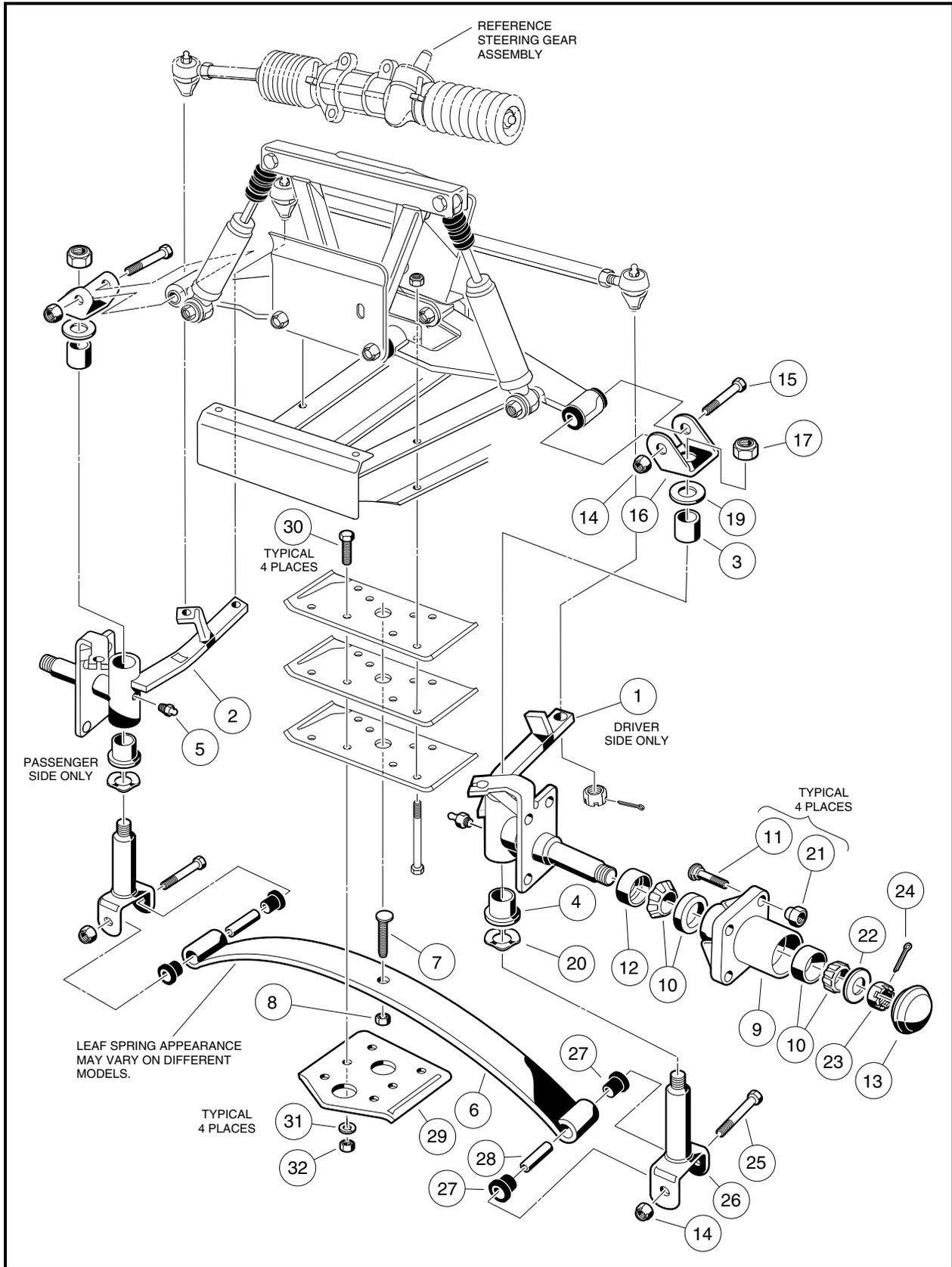
Figure 7-24 Four-Wheel Brake Vehicle – Lower Portion
