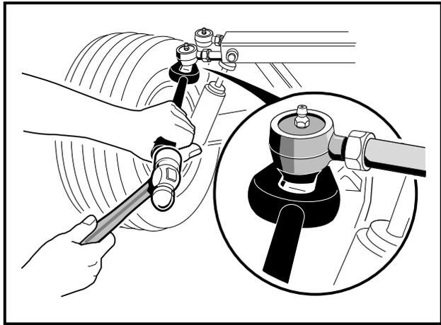
Figure 7-8 Ball Joint Tool
