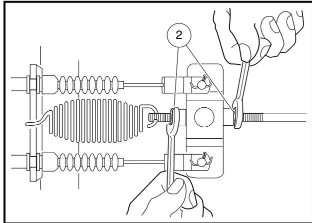
Figure 5-10 Loosen Front Brake Equalizer Rod Nuts
