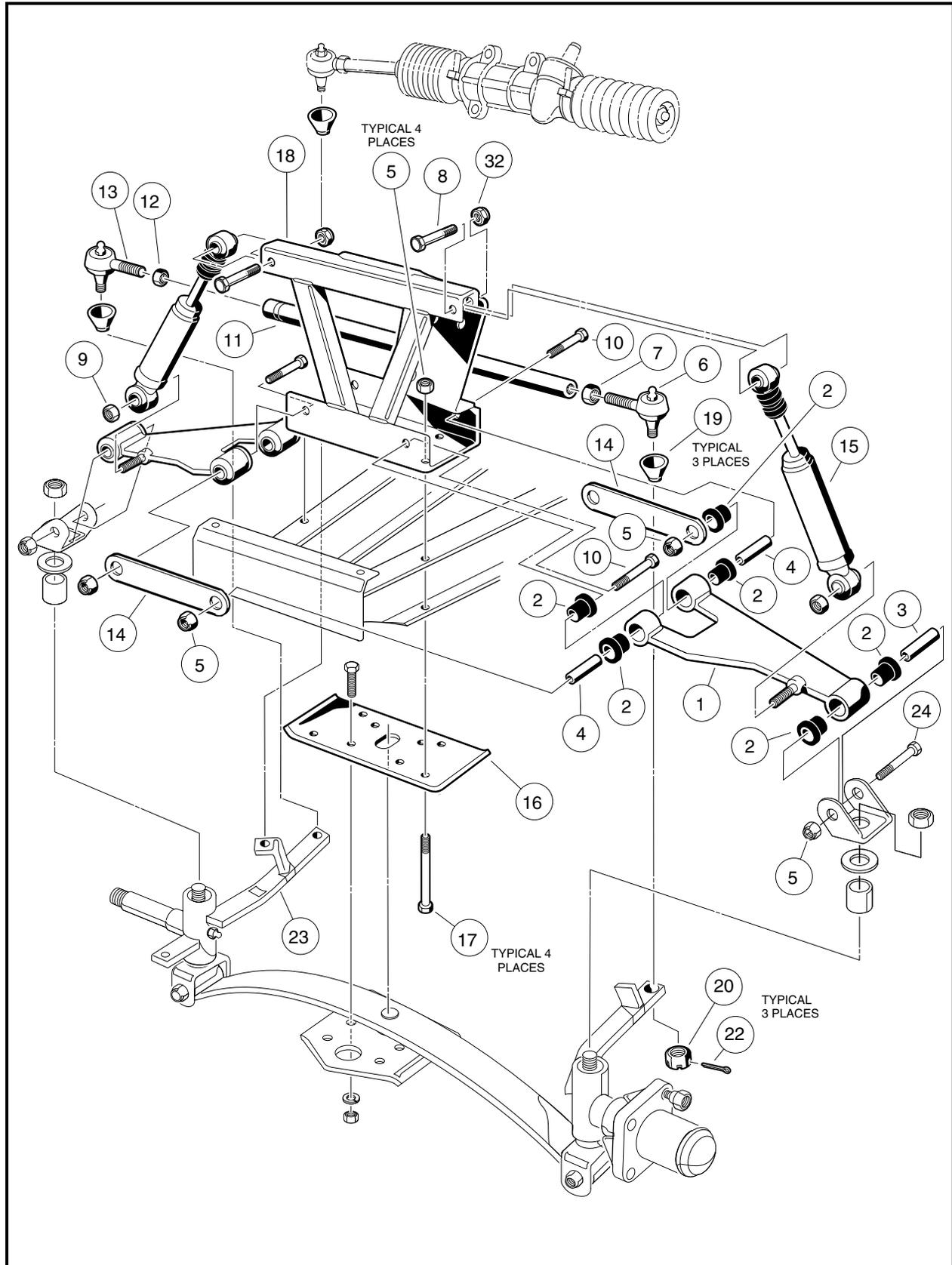
Figure 7-21 Two-Wheel Brake Vehicle – Upper Portion
