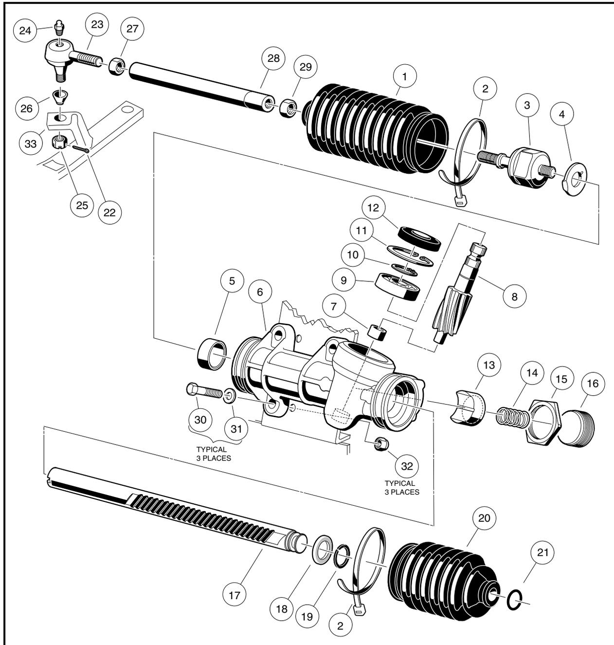
Figure 7-12 Steering Gear
