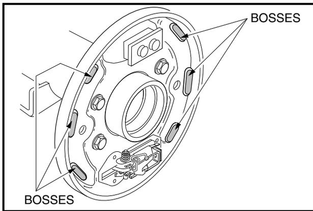
**Figure 6-8 Lubricate Raised Bosses**
