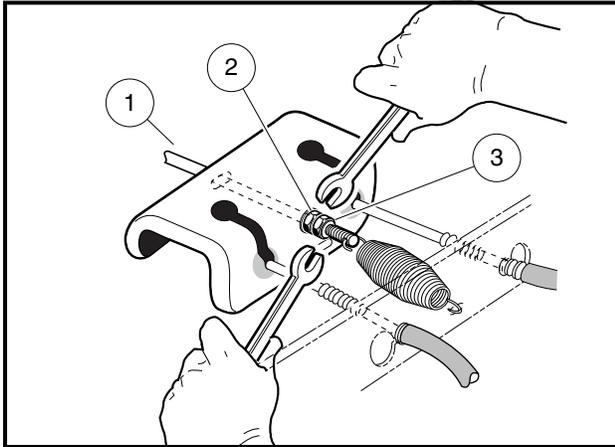
Figure 5-9 Loosen Rear Brake Equalizer Rod Nuts
