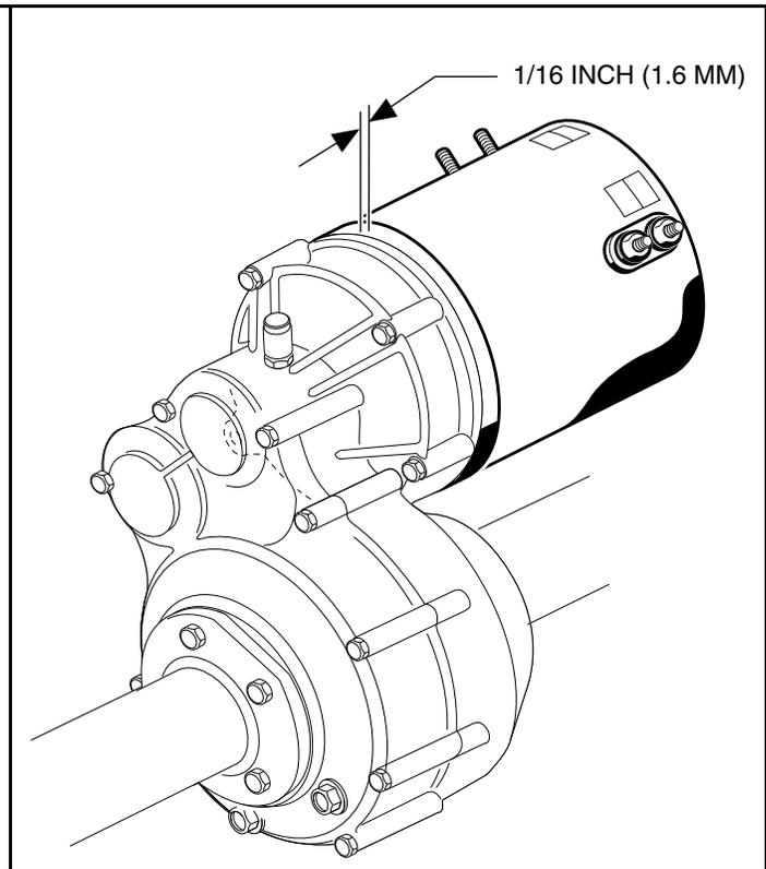
744 **Figure 16-23 Gap at Motor and Transaxle**
