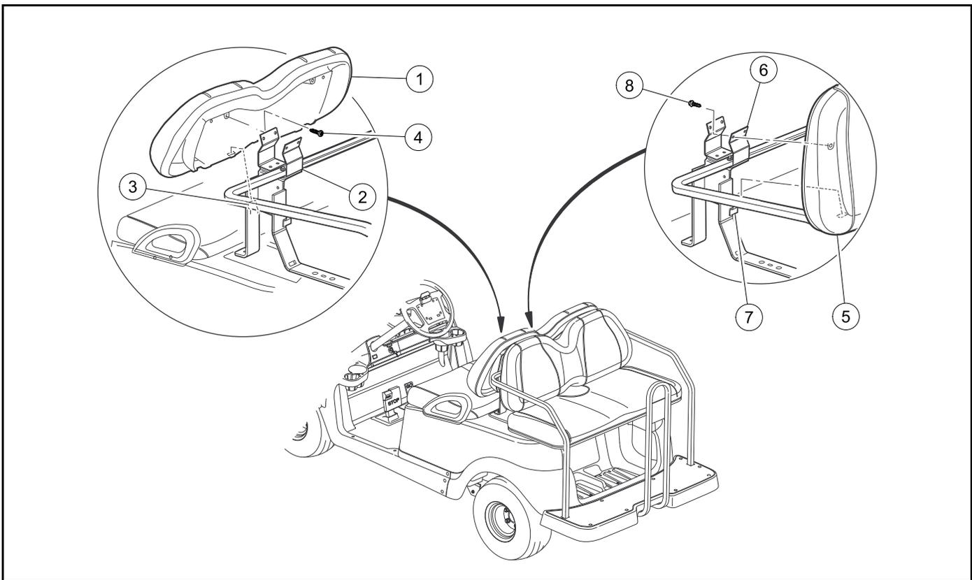
Figure 4-42 Seat Back Installation
