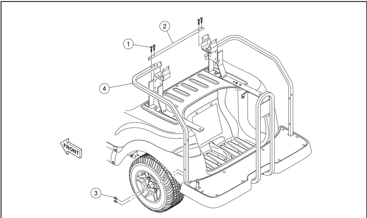
**Figure 4-48 Fold-Down Rear Seat Hip Restraint**
