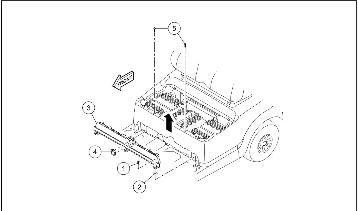
Figure 4-10 Kick Plate and Charger Receptacle Bezel Installation
