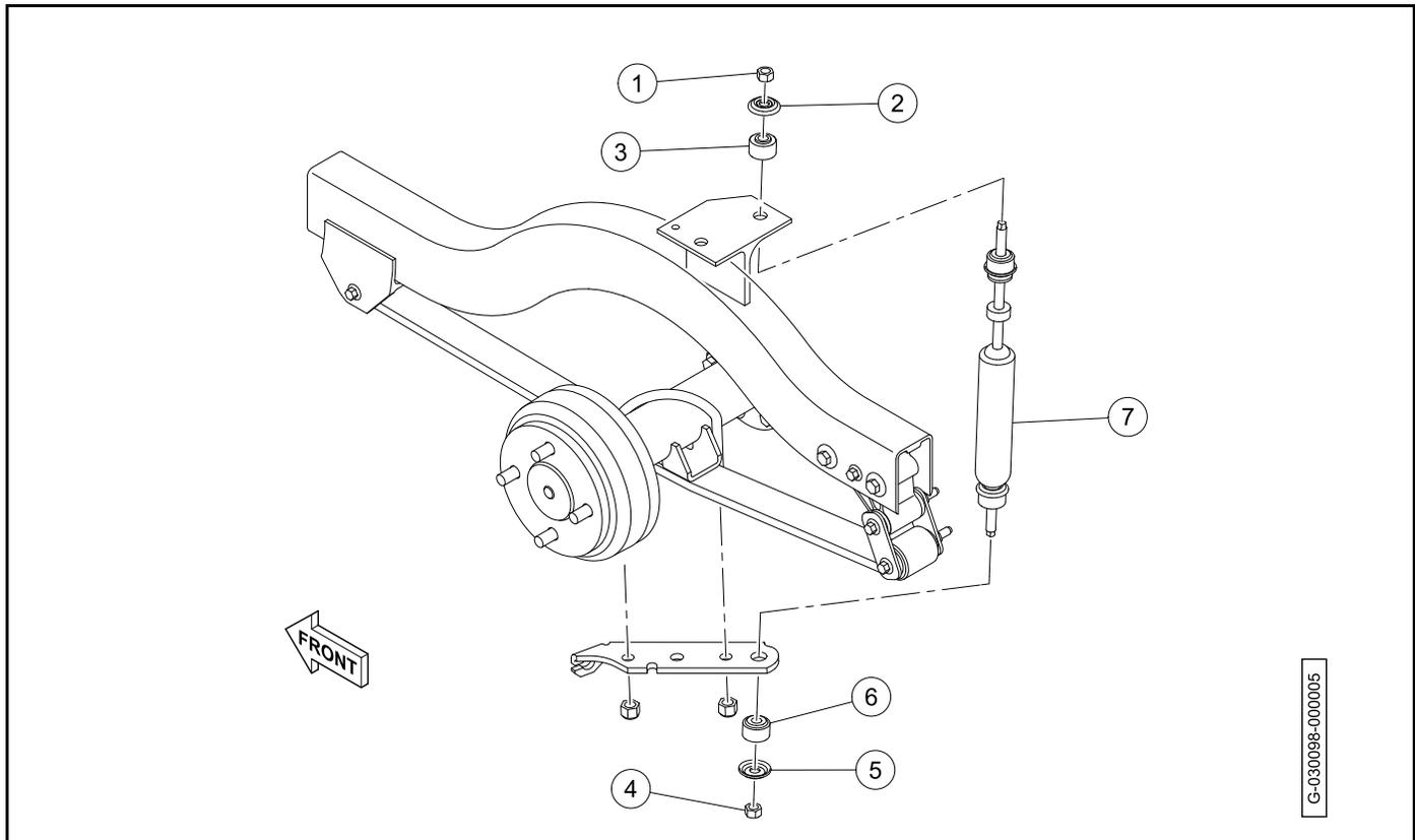
Figure 9-2 Rear Shock Absorber Removal
