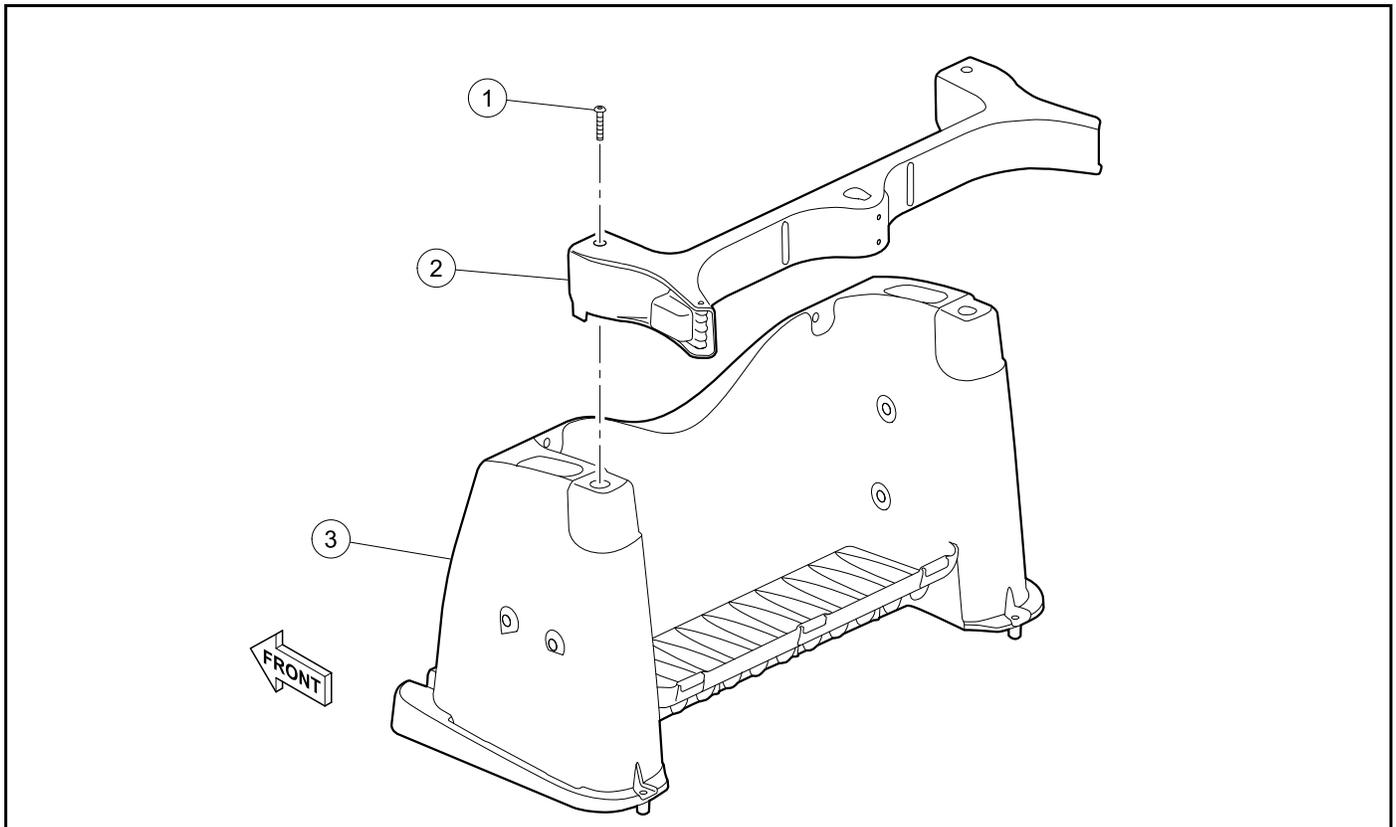
**Figure 4-27 Bag Rack****Bag Rack Removal**
