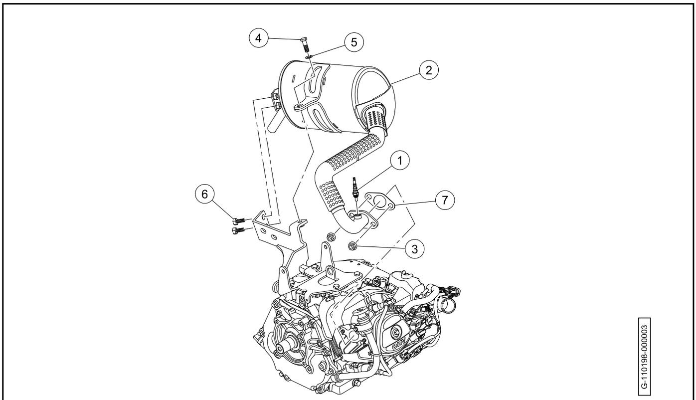
**Figure 22-1 Muffler Removal**
