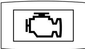
The malfunction indicator light (MIL) gives a visual indication of an engine fault. When the key switch is set to ON, the MIL will turn on for 3 seconds.
