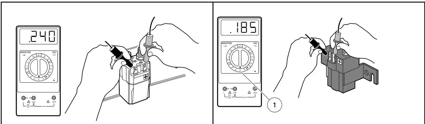
Figure 12-6 Activating Coil Test – Factory-installed Solenoid
