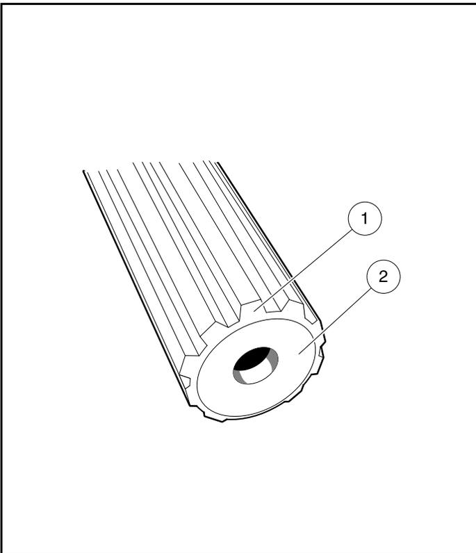
743 **Figure 16-22 Clean Chamfer and Input Shaft End**
