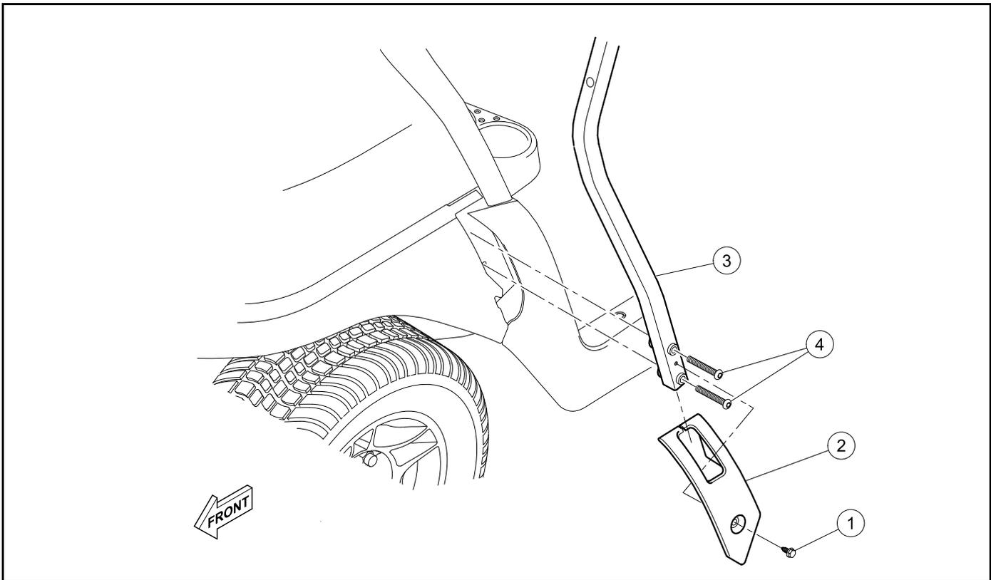
**Figure 4-22 Front Canopy Strut Installation**
