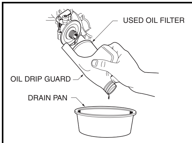
Figure 29 Remove Engine Oil Filter
