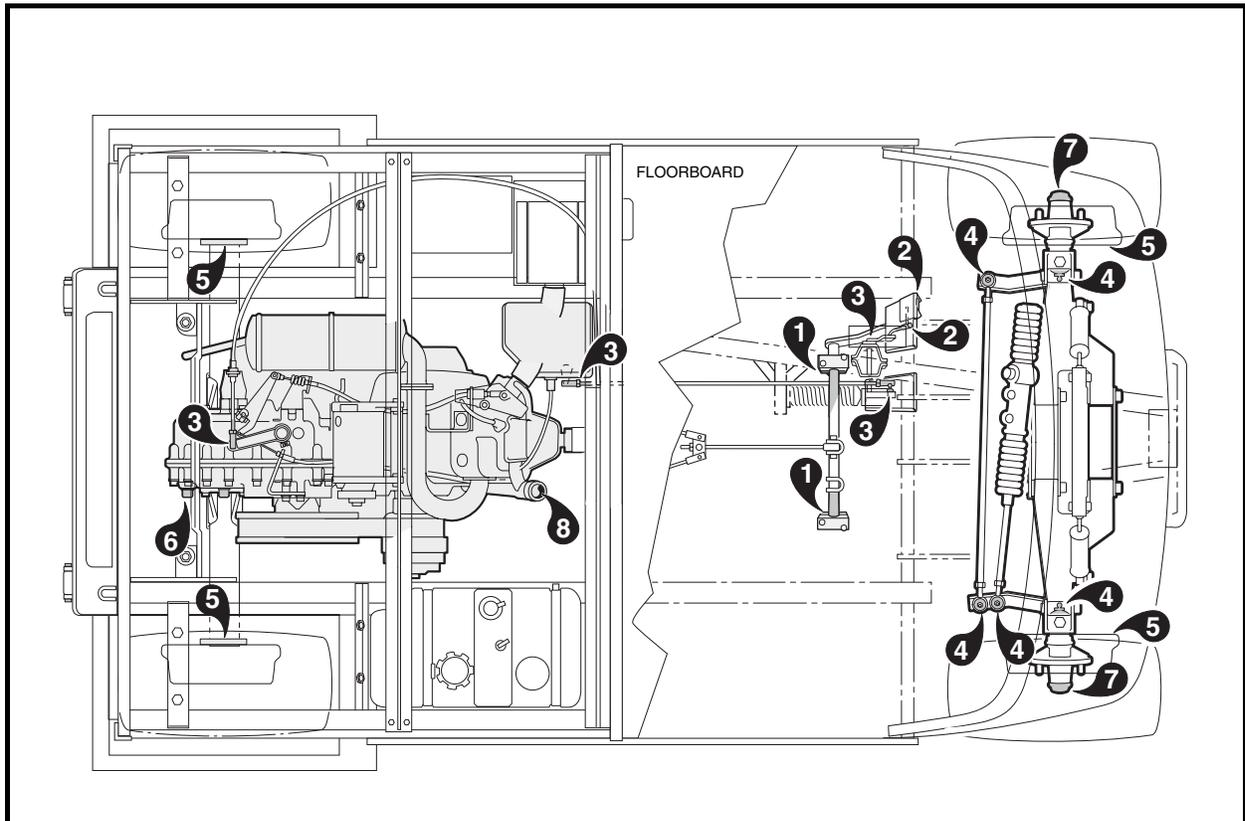
Figure 18 Lubrication Points – Gasoline Vehicles
