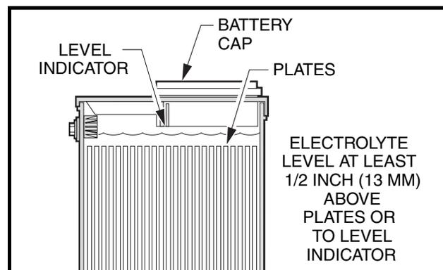
Figure 24 Gasoline Battery Electrolyte Level
