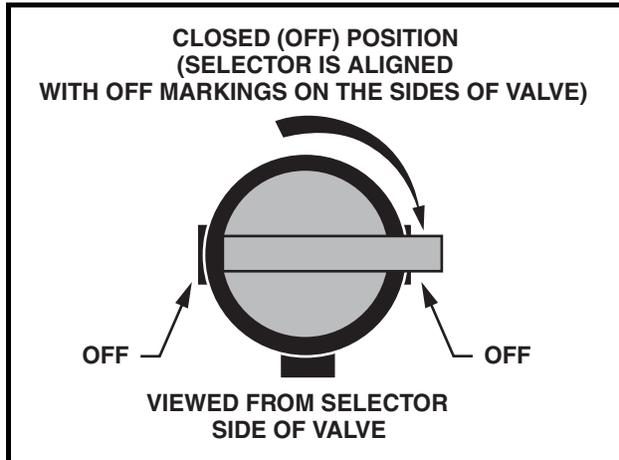
**Figure 14 Fuel Shut-off Valve – Closed Position**
