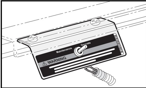
Figure 10 Neutral Lockout Switch
