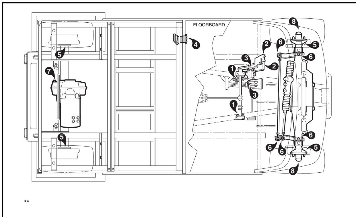
Figure 17 Lubrication Points – Electric Vehicles
